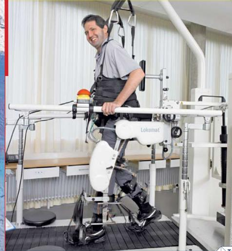
Using technology developed by researchers at the University of Zurich, Hocoma Co. created the Lokomat, the world's first robotic device that automates locomotion therapy on a treadmill and improves the efficiency of treadmill training.
